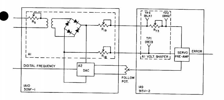
Figure 40-1. Coarse Tune Adjustments
