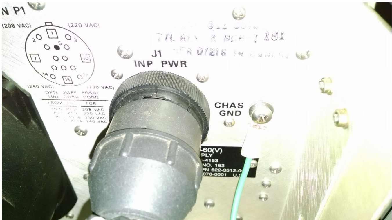
7 - HF-8032 Power Supply, J1 and strapping diagram
