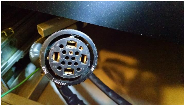
8 - J1 strapped for 208 VAC, pin 5 to pin 2
