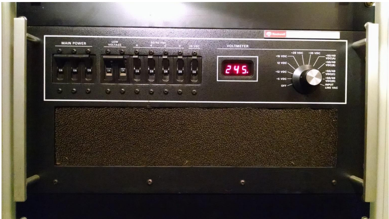
12 - 245 VAC on the incoming line to the HF-8032 PA Power Supply
