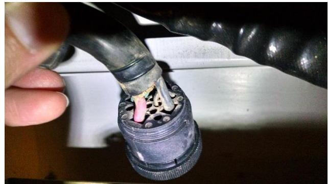
9 - Back side of J1, note strapping jumper
